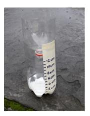
8. At the end of each day, or week, either use the scale along the side of the bottle to take a reading, or pour the resulting water into a measuring cylinder and record your results. These can then be mapped onto a graph (see below), or you could use linking cubes to build towers matching the amounts of rainfall.
